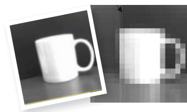
The images above demonstrates how information from the camera is represented on the tongue. Left image: camera image; Right image: Graphic rendering of the tongue display.
